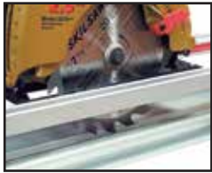
Recessed saw blade track to avoid tabletop cut through
