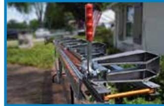
Easy to use, positive toggle lock with single point adjustment.
