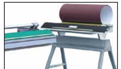
Allows material to be fed directly into brakes or slitters.
