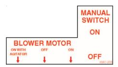
Specifies the manual switch (Bypasses remote) and indicates if the blower is off, on, or on with agitator.
